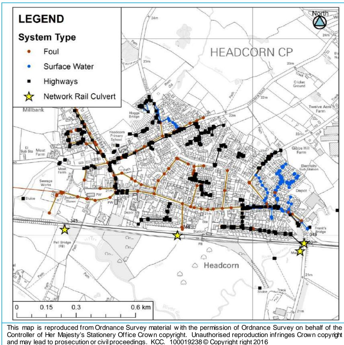
Figure 3-5 Headcorn urban drainage network
