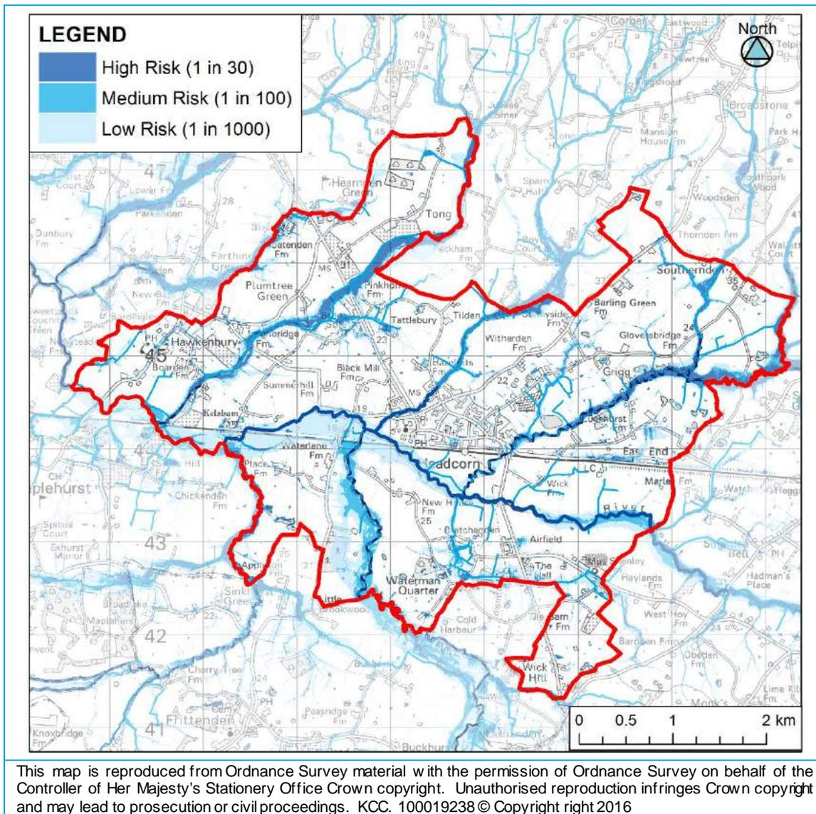
Figure 3-7 High, medium and low surface water flood risk in Headcorn according to the uFMfSW
