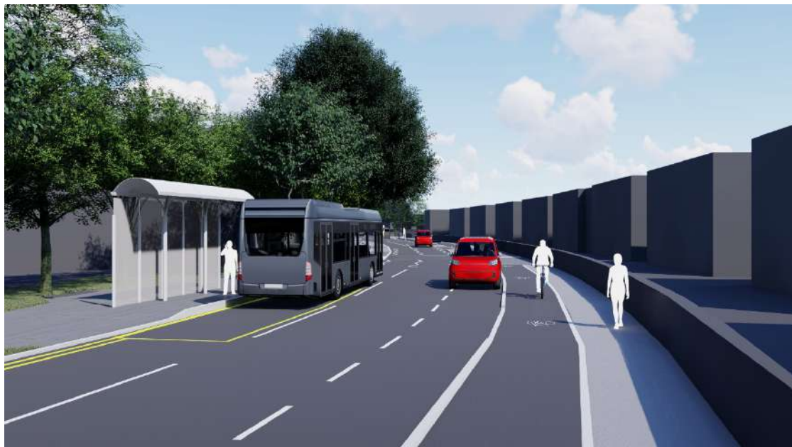
Visualisation 3 (right): Shows a southbound fully segregated stepped cycle track and a northbound bus stop with shared pedestrian and cycle footway to allow passengers ease of access to buses. Signage will support the shared cycle/pedestrian areas to provide safety and minimise conflict between pedestrians and cyclists.
