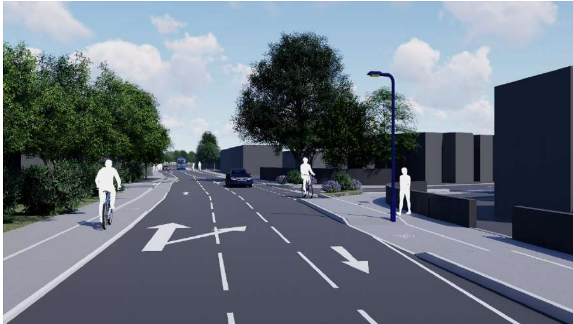
Visualisation 2 (left): Proposed layout of Springhead Road. The visual shows where cyclists would be accommodated within the fully segregated stepped cycle track and the widening of the footway where possible to make it more accessible to improve pedestrian safety.
