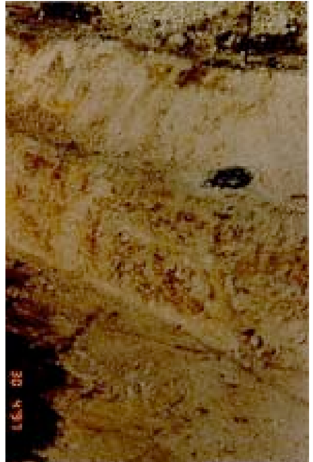
Plate 6 Orange iron-staining to chalk close to a solution feature
