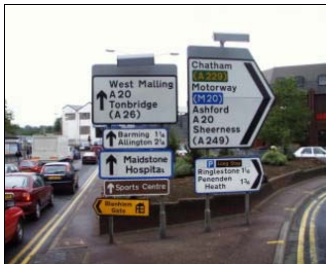
Signing strategies can reduce tendency for sign structures to have an uncoordinated appearance through successive add-ons
