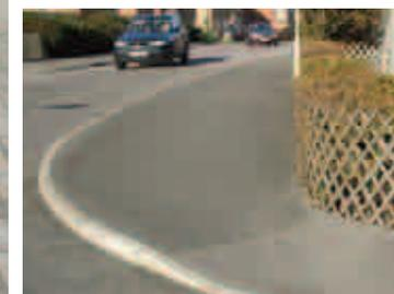
In an urban or suburban setting, the footway normally defines the visibility splay characteristics (top right).
