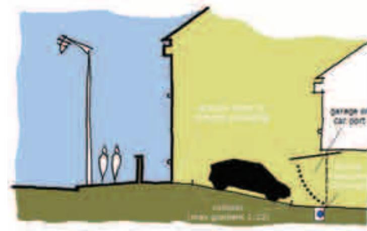
Roads must either have a cross-fall or cambered profile, generally with a gradient of 2.5% (1 in 40).
