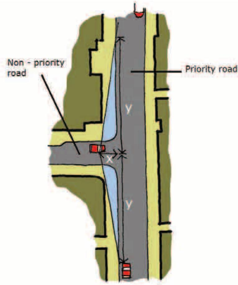
Forward visibility is normally measured between points in the road 1.5m from the channel line. (further information about how to measure visibility is provided in 'Design Bulletin 32 – Residential Roads and Footpaths', published by the Department of Environment and Transport)
