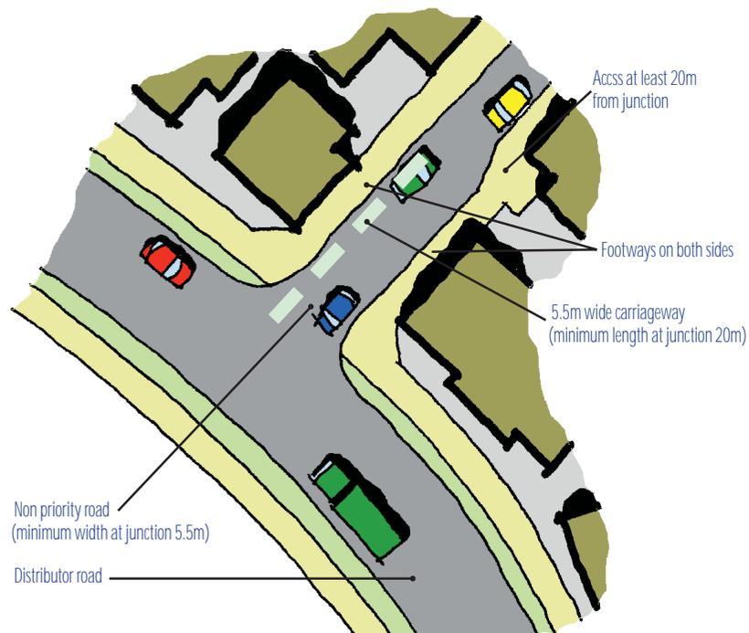
Junction arrangements involving major alterations to the existing highway are covered by separate agreements under Section 278 of the Highways Act 1980.
