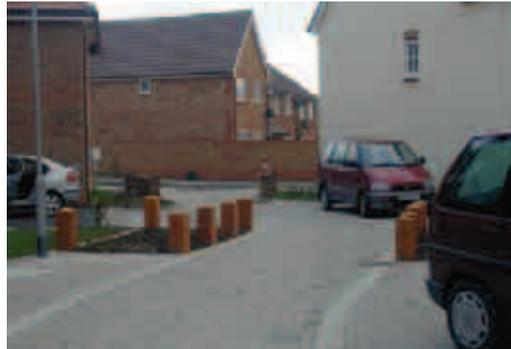
A combination of building layout, parking and street furniture can help define a safe vehicle path through a development. Use of materials for a carriageway surface can help define different areas.
