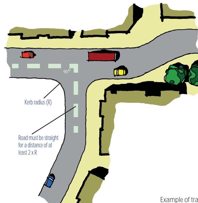
Example of traditional T-Junction with short length of straight before a curve (below).
