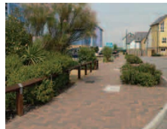
Where an emerging vehicle needs to cross a footway or service margin from a shared or individual private driveway, pedestrians and cyclists must be given sufficient warning of the vehicle's approach. In such circumstances a visibility splay of 2mx2m is required from the back edge of the highway limit as shown (below and right).
