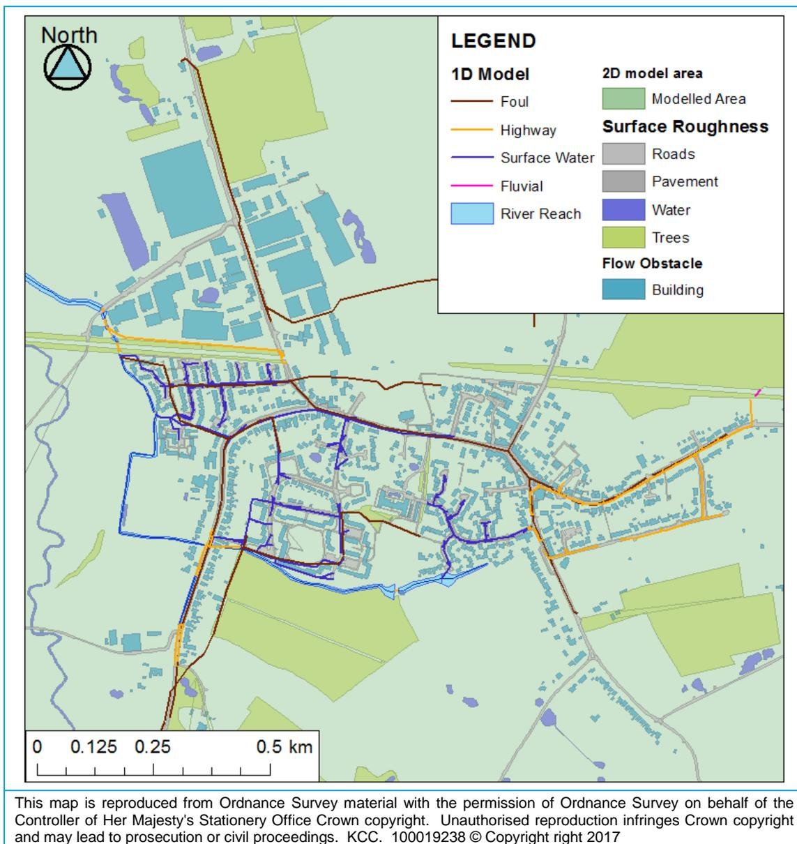
Figure 3-8: Marden IUD model schematic
