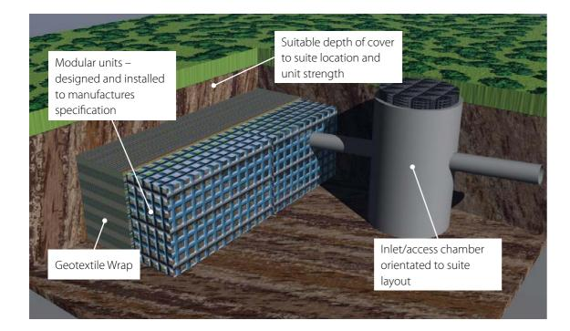
Image F.1 – example of a modular cell filled trench soakaway (WSP)
