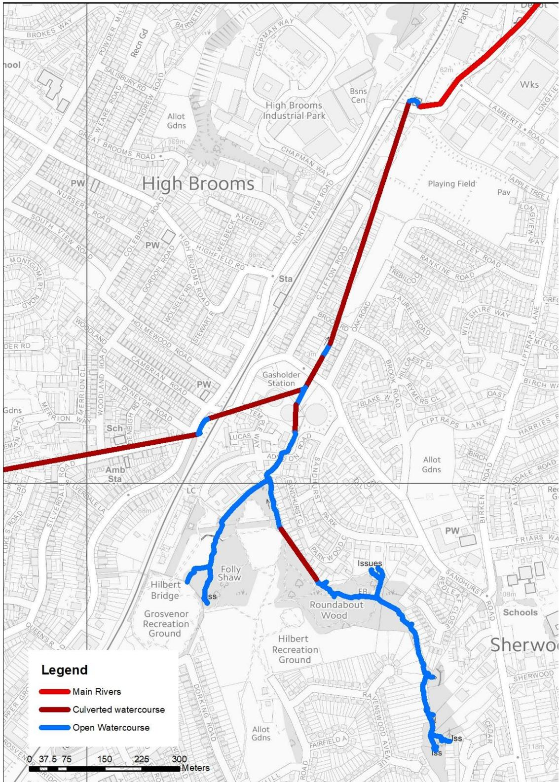
Figure 7 Approximate location of culverted sections of the Southborough Stream
