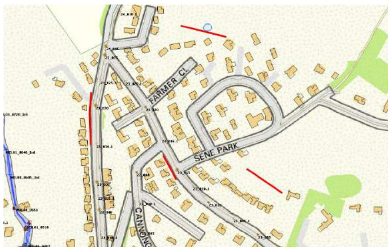
Figure 3-6: Schematisation of flow diversion bunds at Sene Park
