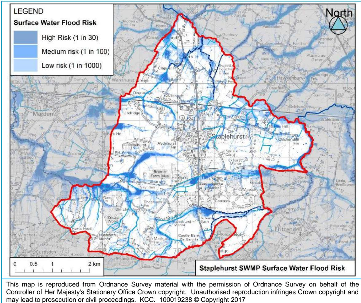
Figure 3-7 High, medium and low surface water flood risk in Staplehurst according to the uFMfSW
