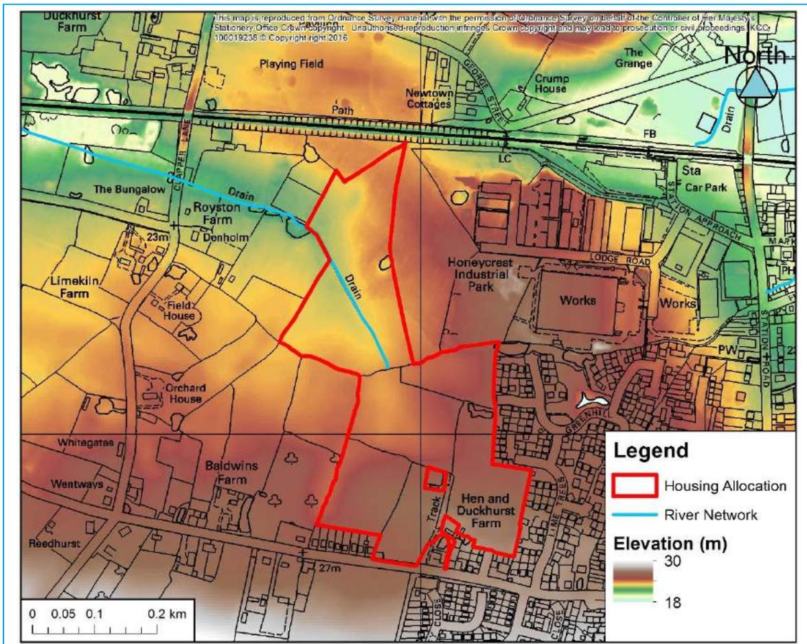
The development site is directly adjacent to Marden Road which is one of the flooding hotspots identified in Staplehurst. Due to the lie of the land, surface water from the development would drain away from Marden Road and should not increase surface water flooding, but the site itself could be at risk of flooding from Marden Road.
