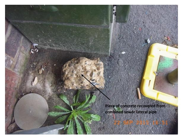
Photo 2 Piece of concrete recovered from 150mm diameter combined sewer line (Source: Southern Water)
