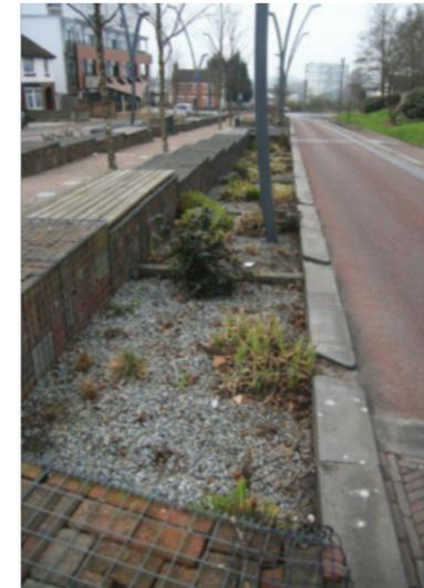
**Photo G.3** – typical example of Bioretention area (Source: Susdrain)
