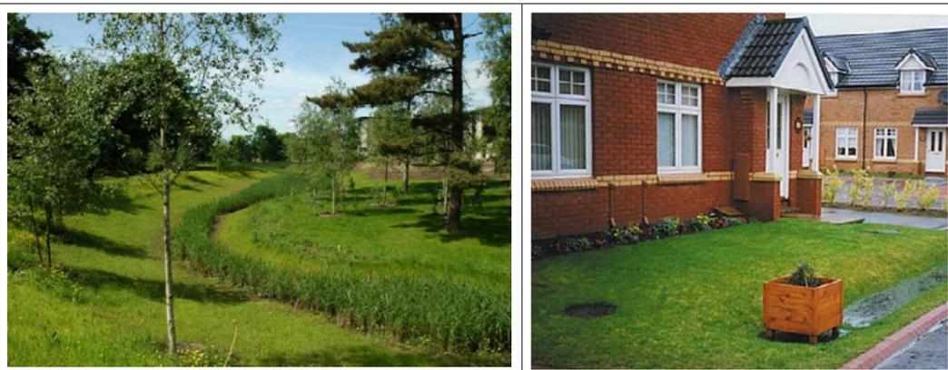
Photos E.1 and E.2 – example of a large scale swale (left) and small scale swale (right)
