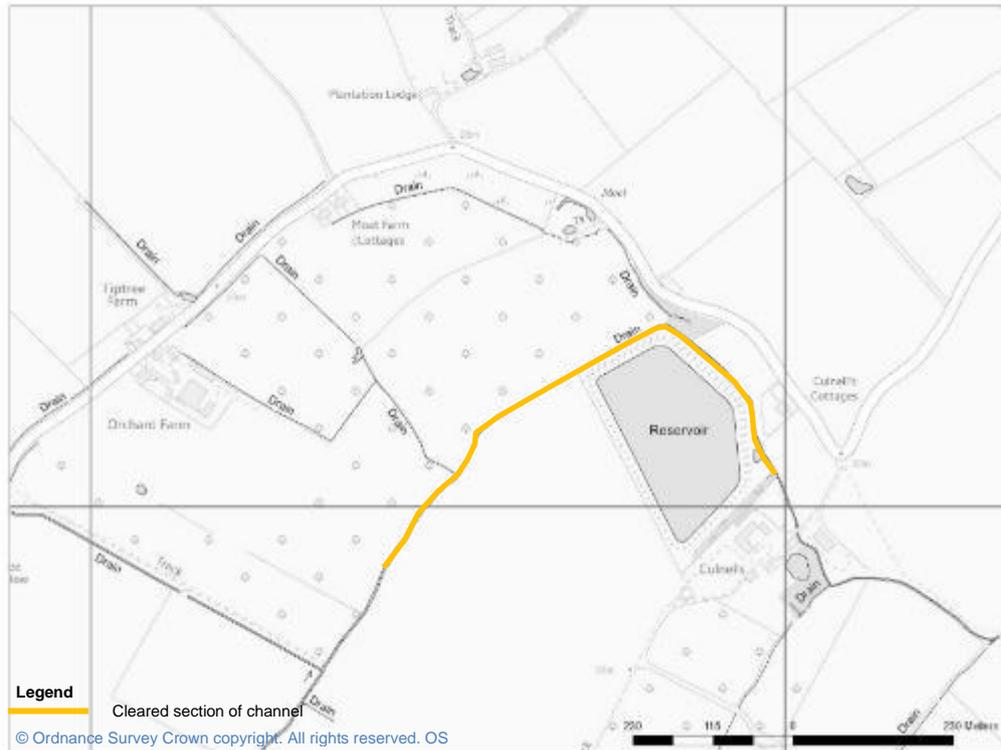
**Figure 8 Location of clearance work along Iwade Stream**
