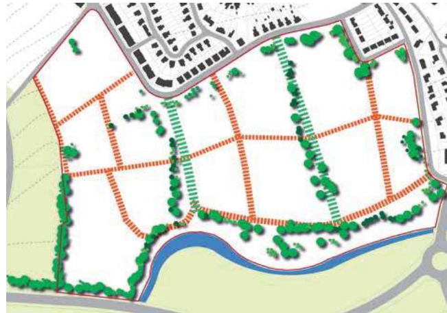
Street structuring for gravity surface drainage
