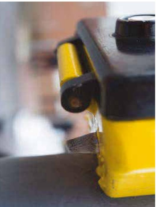
The 'spinning cone' that rotates when the Green Man shows.
