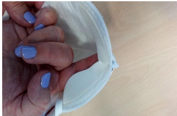
Photo 2: Non defective mask: no gap between nose band and respirator
