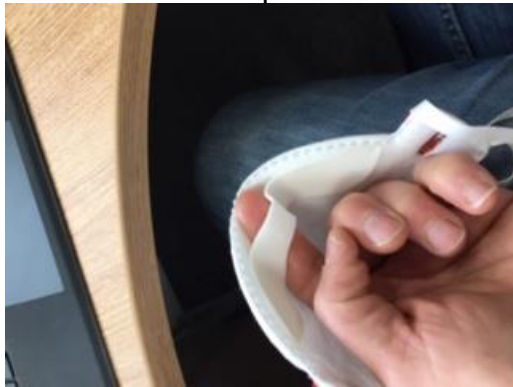
Photo 1: Defective mask: gap between nose band and respirator
