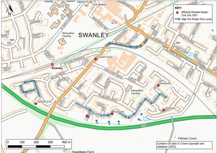
Figure 6 - High Firs Estate Flood Mechanisms
