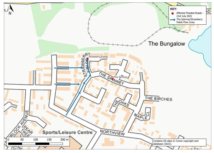
Figure 8 - The Spinney / Strawberry Fields flood mechanisms
