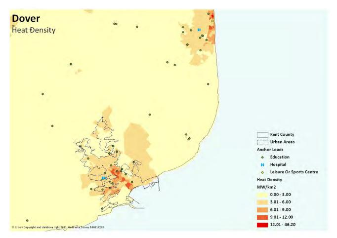
Figure 34: Heat map for Dover
