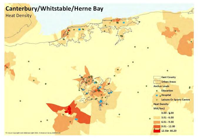
Figure 32: Heat map for Canterbury/Whitstable/Herne Bay<sup>21</sup>
