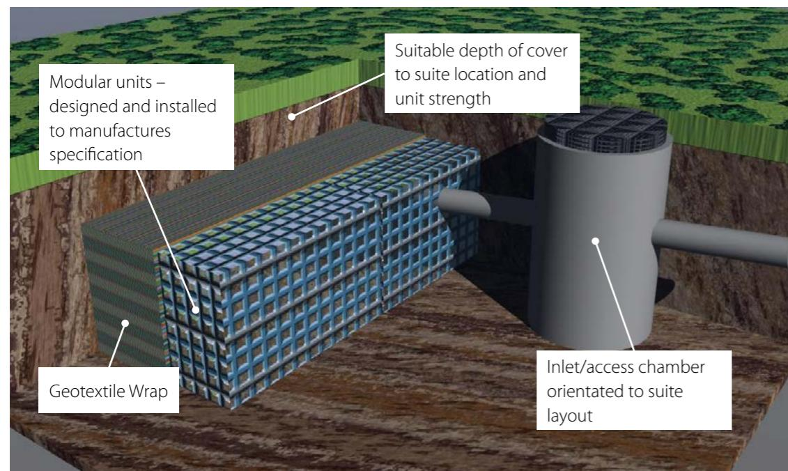
**Image F.1** – example of a modular cell filled trench soakaway (WSP)
